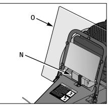
Figure 2-5: Lift and tilt debris shield forward to locate battery.
